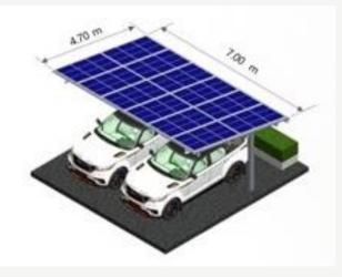
2 car parking 12 panel solar roof Dimensions 7.00m wide x 4.70m deep Inside pole dimensions 5.70m. Solar panel size 1,134 x 2, 261 x 35 mm. Size 550 Wp/panel. 12 panels = 6.60 kWp.
