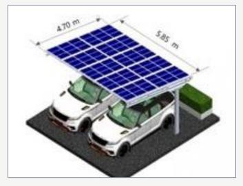
2 car parking 10 panel solar roof Dimensions 5.85m wide x 4.70m deep Inside pole dimensions 5.50m. Solar panel size 1,134 x 2, 261 x 35 mm. Size 550 Wp/panel. 10 panels = 5.50 kWp.
